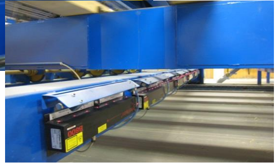
ROSGRADE STRENGTH GRADING MACHINE NATURAL FREQUENCY
