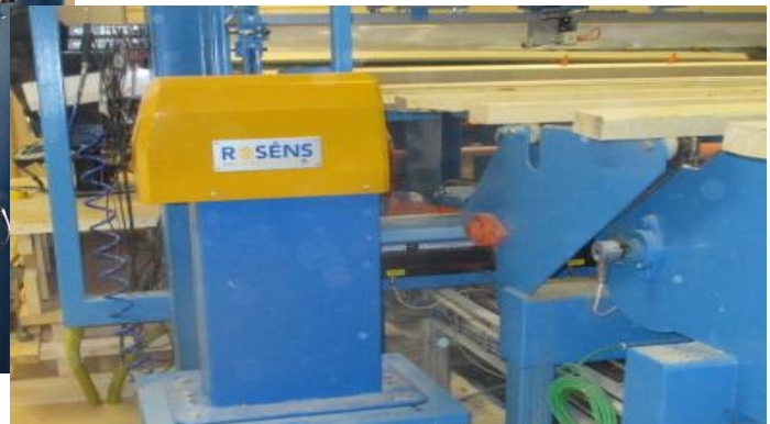
ROSGRADE STRENGTH GRADING MACHINE NATURAL FREQUENCY
